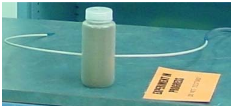
Figure 8. The Moisture Evaporation Tube for the Fiber Sensor, soon to be Buried
