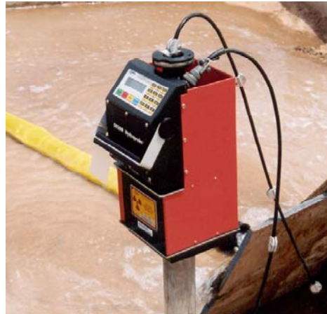
Figure 1. Neutron Probe Monitoring Soil Moisture
