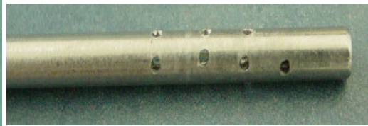
Figure 2: The holes are over the relative humidity grating
