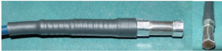
Figure 3: Side and end views of the moisture sensor housing
