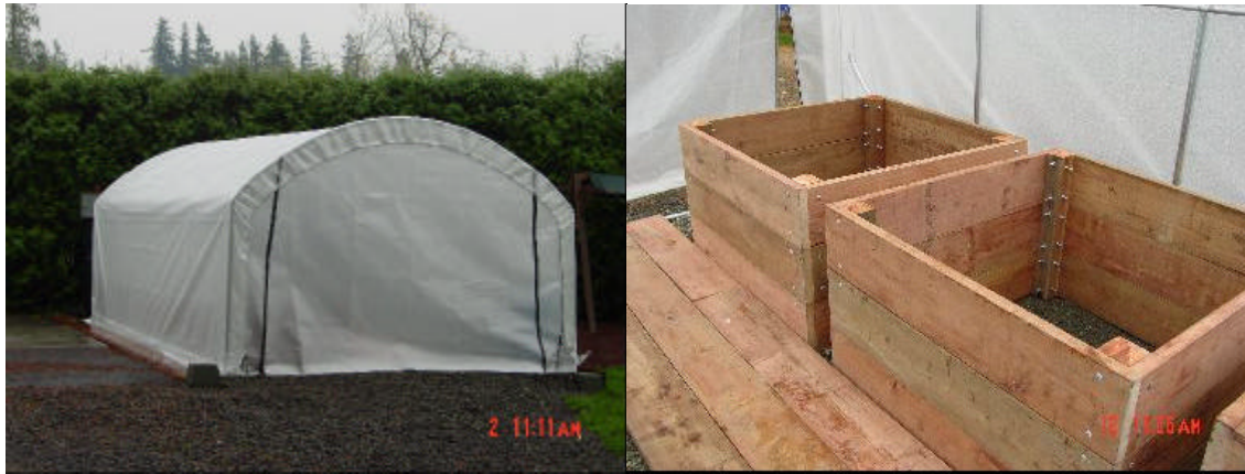
Figure 14: Blue Road Research soil moisture testing facility: a) greenhouse and b) soil test boxes
