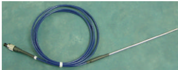
Figure 1: The probe for measuring temperature and relative humidity
