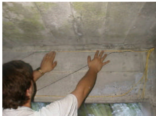
Figure 2. 1.0 m fiber grating sensors used to support multipoint, high-speed dynamic strain measurements.
