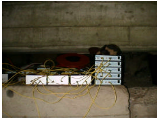
Figure 4. Five high-speed, high-sensitivity fiber grating demodulation systems used by Blue Road Research for measurements.
