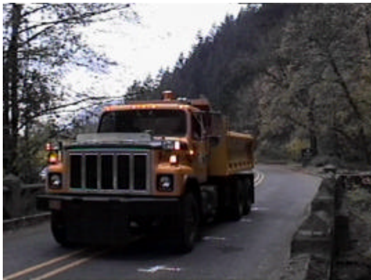
Figure 3. Test vehicle used for static and dynamic testing of the Horsetail Falls Bridge.
