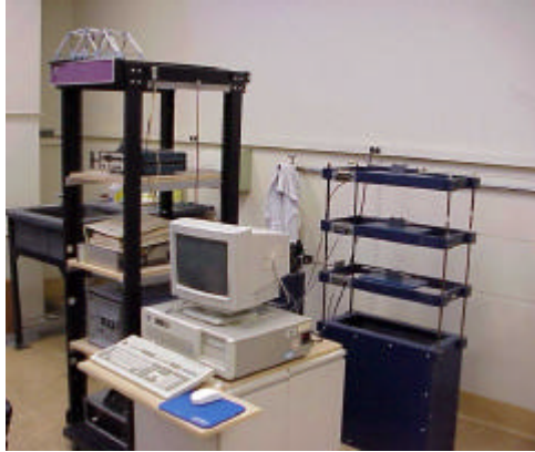
Fig. 10 Shaker table setup (left) and structural models (right) of forced vibration tests
