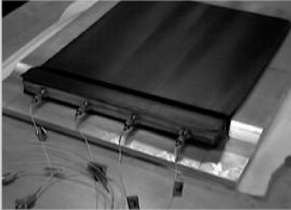
Figure 5. Carbon epoxy panel with four embedded multi-axis fiber grating strain sensors to measure transverse, axial and shear strain.
