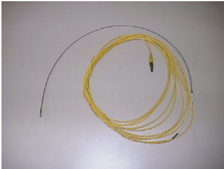
Figure 3: A 70cm gauge length fiber optic strain sensor and cable.
