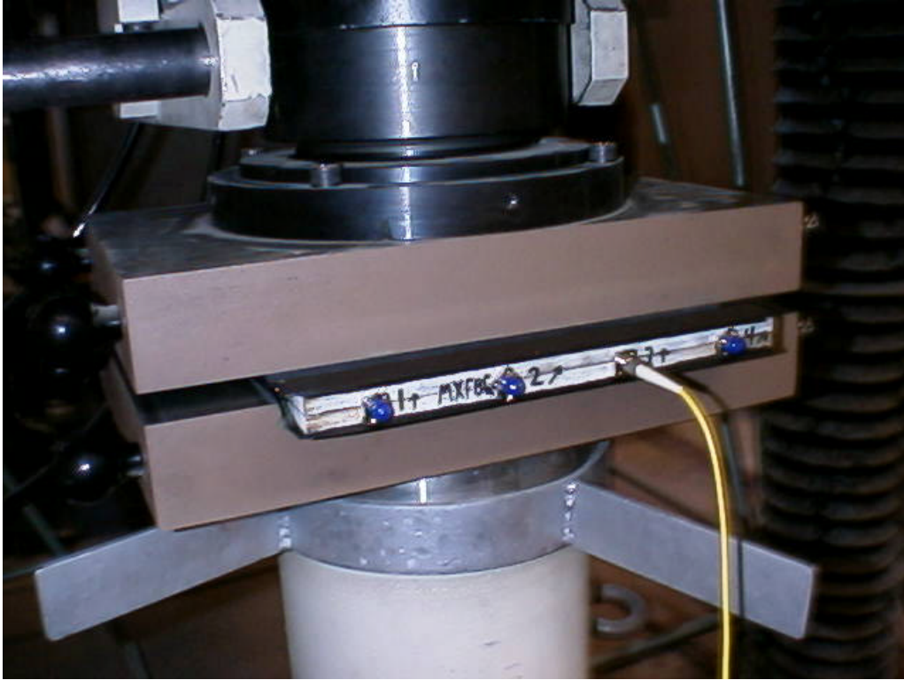
Figure 6. Load testing of composite load cell with embedded multi-axis fiber grating strain sensors
