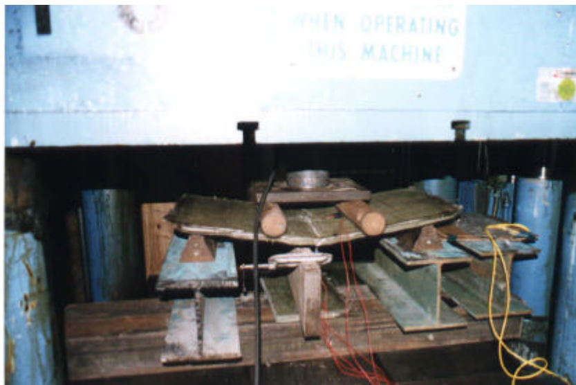
Figure 6: Composite panels with embedded grating sensors were used in drop tests (see Figure 6) and three point bend tests (shown here).
